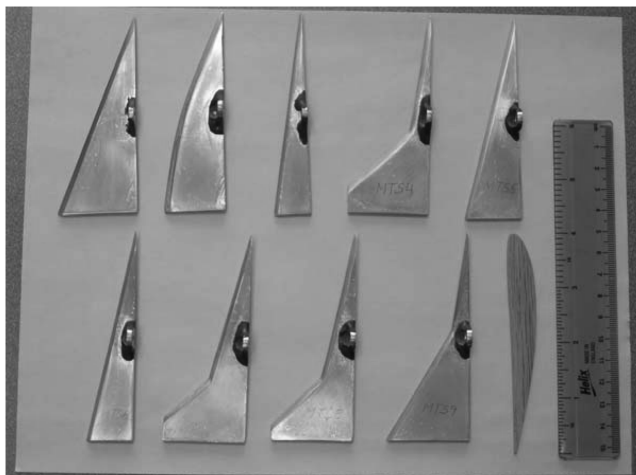
Fig. 1 Port (left) halves of nine models of movable tip strakes: MTS1–MTS9 (from left to right and top to bottom).
